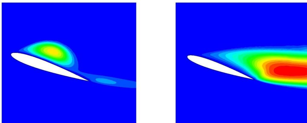
**Figure 6: Turbulent nu term at 19.24 degrees on the upstroke (left: unsteady, right: quasi steady)**
