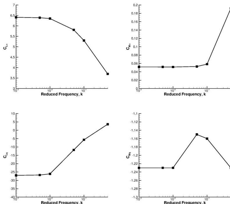
**Figure 10: Variation of dynamic derivatives with reduced frequency**
