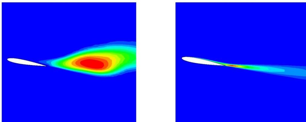
**Figure 7: Turbulent nu term at 10 degrees on the downstroke (left: unsteady, right: quasi steady)**
