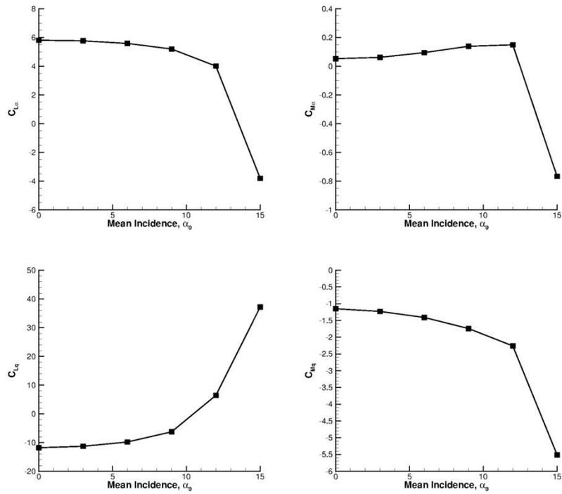
**Figure 8: Variation of dynamic derivatives with mean incidence**
