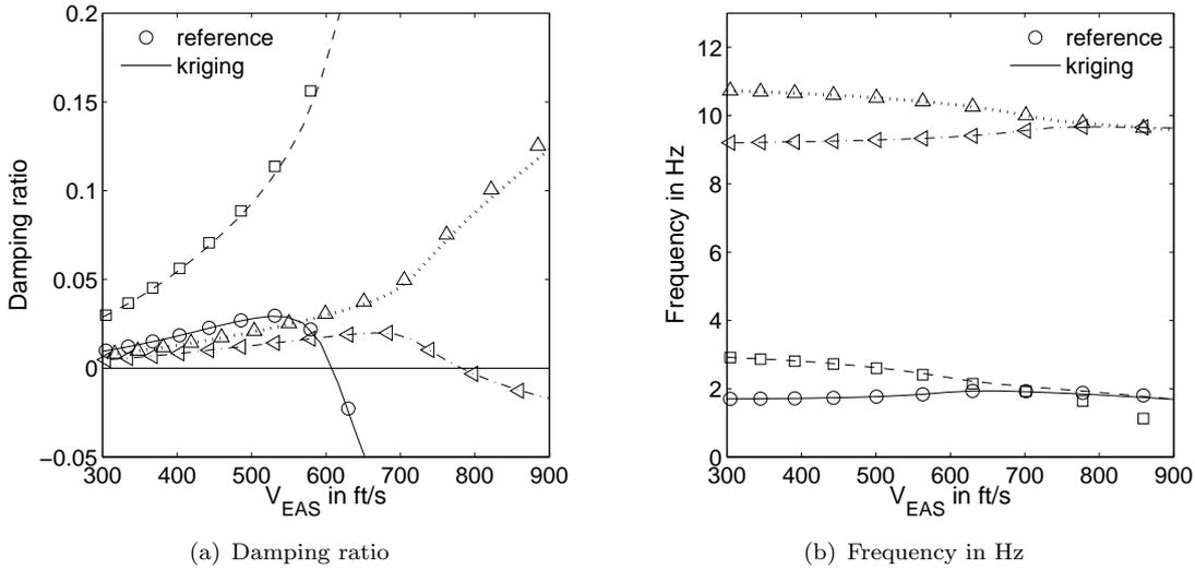
Figure 5. Damping ratio and frequency vs. equivalent airspeed (VEAS) for Goland wing/store configuration.
