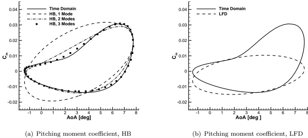
Figure 6. NACA 0012: pitching moment coefficients dynamic dependence ( $M = 0.6$ ,  $\alpha_0 = 3.16^\circ$ ,  $\alpha_A = 4.59^\circ$ , and  $k = 0.0811$ )
