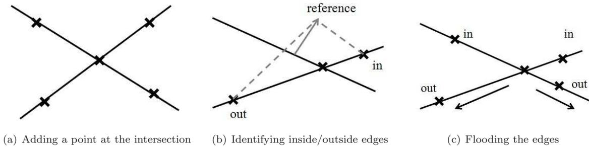
Figure 14. Boundary intersection diagrams
