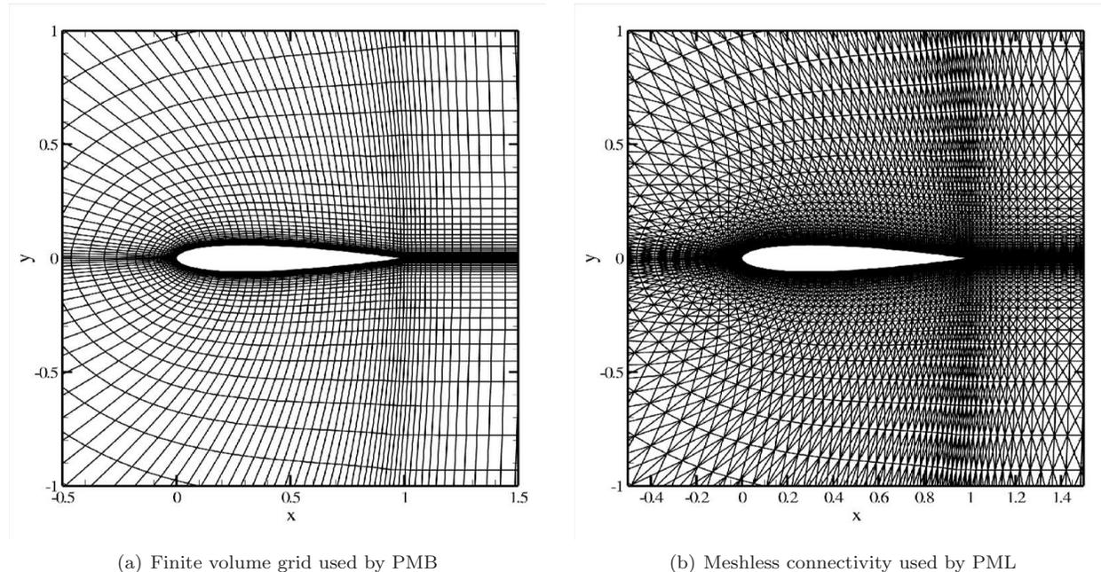
Figure 2. NACA0012 aerofoil used for 2D calculations
