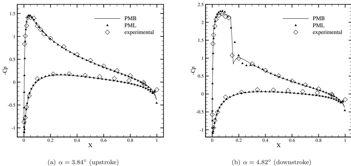
Figure 9. Unsteady pressure distributions for forced pitching motion test case of AGARD CT1
