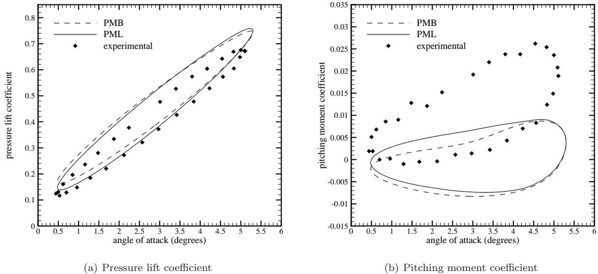
Figure 8. Lift coefficients for moving NACA0012 aerofoil
