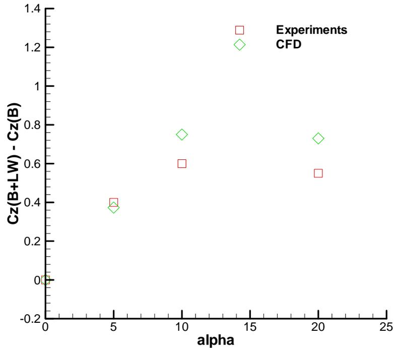
Delta on the normal force due to the lattice wings.
