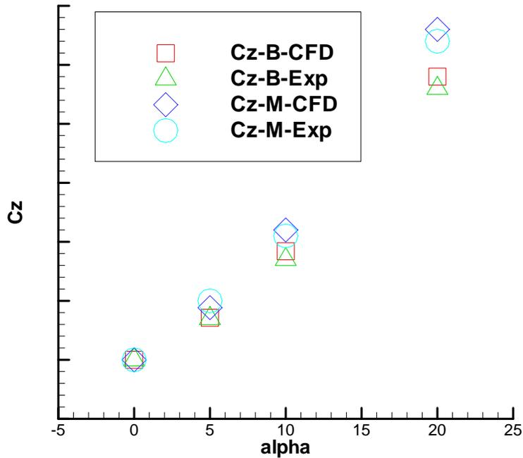
Experimental and numerical values of the normal force coefficient at Mach 4.
