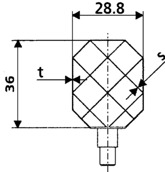
$$\begin{aligned}s &= 0.30 \text{ mm} \\t &= 0.30 \text{ mm} \\s_z &= 891 \text{ mm}^2 \\s_y &= 958 \text{ mm}^2 \\s_x &= 85 \text{ mm}^2\end{aligned}$$
