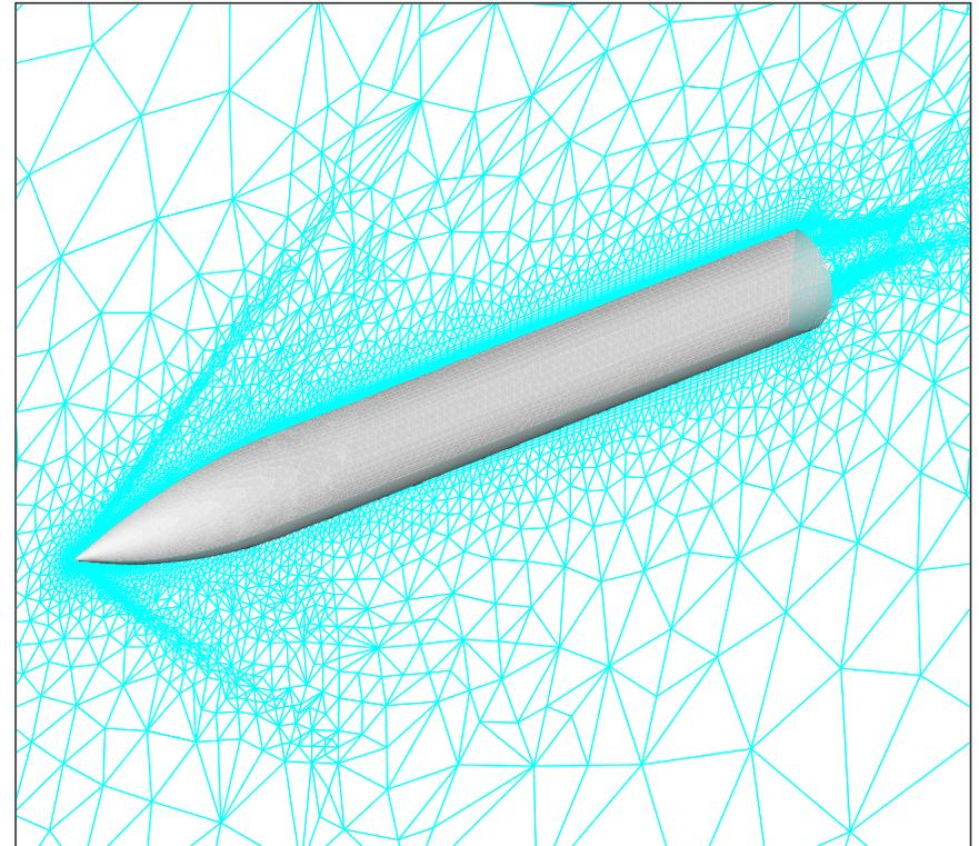
Mesh used for the body: symmetry plane along the vehicle.
