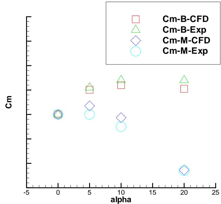
Experimental and numerical values of the pitching moment coefficient at Mach 4.
