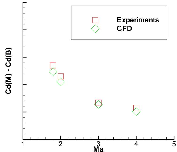
Delta on the drag due to the lattice wings.
