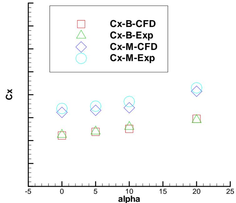
Evolution of the axial force coefficient with the angle of attack at Mach4
