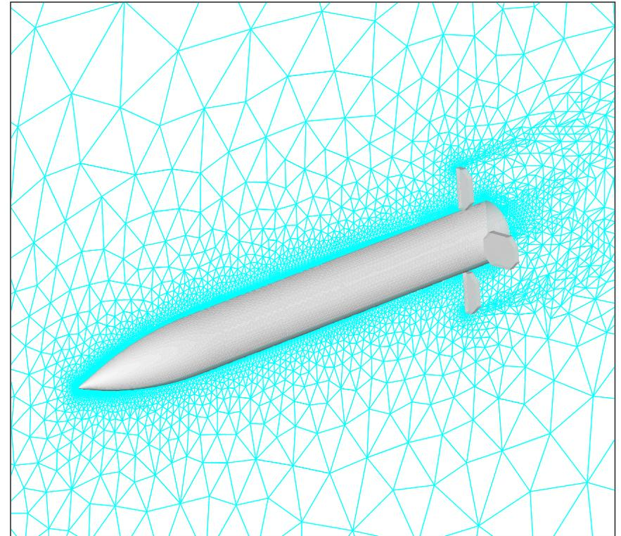
Mesh used for the complete vehicle: symmetry plane along the vehicle.
