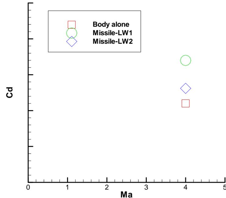
Effects of the grid fin geometry on the drag at Mach 4 (LW1: thick grid fin, LW2 thin grid fin).
