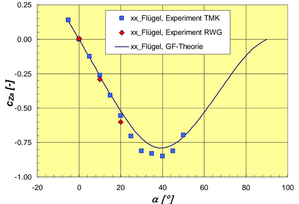
**Validation of lattice wing theory at Mach 3 with experimental data for a XX-grid fin: Comparison of the theoretical axial force coefficient against TMK– and RWG – measurements.**
