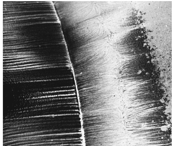
Fig. 5 : 3D micro structures in an axisymmetric reattachment region
