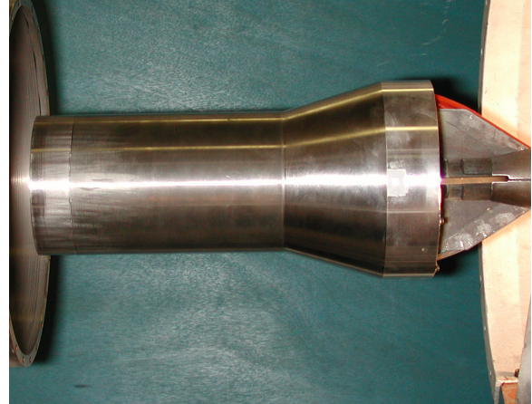
Fig. 4 : Hollow cylinder-plus-flare model for axisymmetric flow investigation
