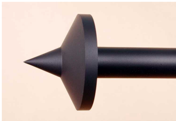
a – double cone model for hypersonic separation study
