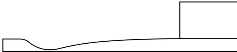
Figure 9: H3 nozzle geometry
